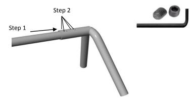
To assemble 17'1" top rail take the 11'7" top rail and the 5'6" top rail with welded 1 7/8" pipe. Sleeve the 18" of 1 7/8" into the 11'7" top rail. Now that you have it sleeved all the way in, secure it by using 2-3/8" set screws and securing them tight (with allen wrench provided) in the 2 holes drilled and tapped at the top of the 11'7" top rail.
