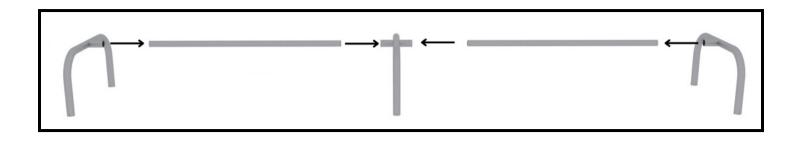
**Step 3**: Insert and tighten (4) 3/8" x 3/8" set screws into each of the Arch Sleeves using the allen wrench provided. Tighten as hard as you can, but do not use power tools to do this!
