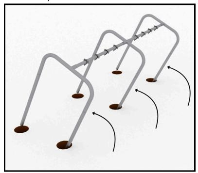
5. Place a level on the top rail and make the necessary adjustments to get the structure level.
