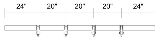
**Step 2**: Slide the ends of the 9' Top Rail as far as they will go into the Sleeves of the Arches.
