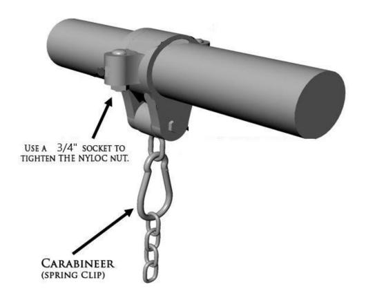
1. Loosen and remove the two nylock jam nuts. 2. Reassemble on to swing top rail. Tighten securely so that the hanger is
