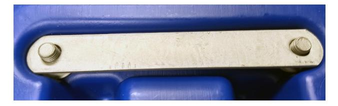
**Step 3** - Place the washer and lock nut over the threads and begin tightening with a socket wrench. Tighten down a few turns on one side and switch to the other side and keep repeating this. This should force the cross plate down into the plastic. Once the cross plate is nearly down as far as it can go, you can stop ratcheting.
