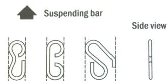
Acceptable S-hook orientation
